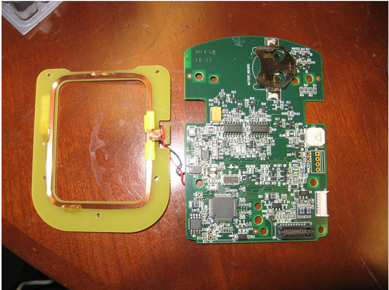
Backside of 125KHz Radio Board with Antenna
