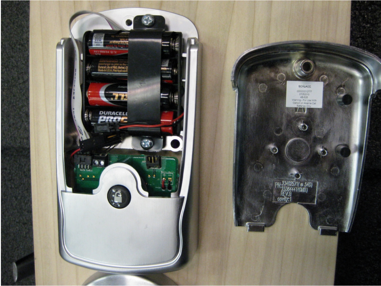
Backside of Door Cover removed
