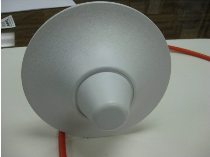
Front side of Dome Antenna
