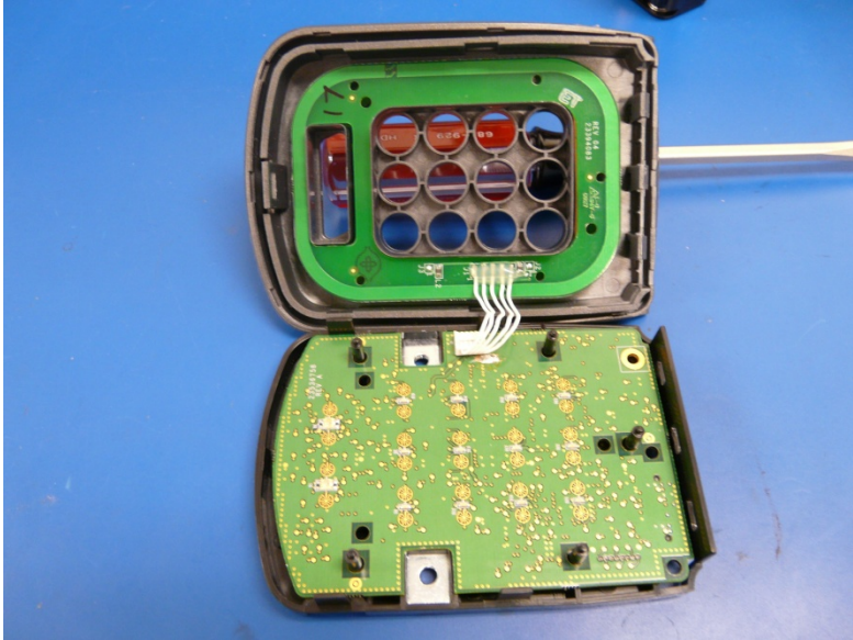
Open for Inspection-Backside of RF Section, View #1
