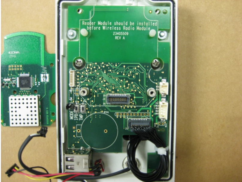
Internal Photo that contains certified 900MHz RF Module removed
