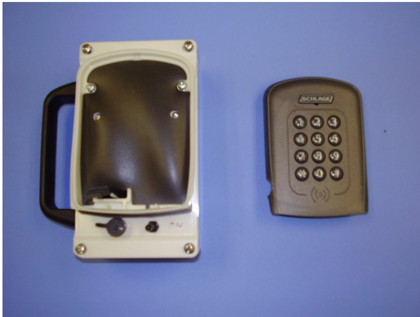
View with Multi-tech and Smart Card Reader Removed
