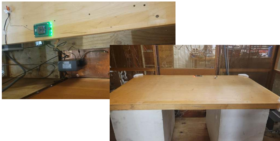
Figure 6: Conducted Emissions Test Setup Photograph(s).
