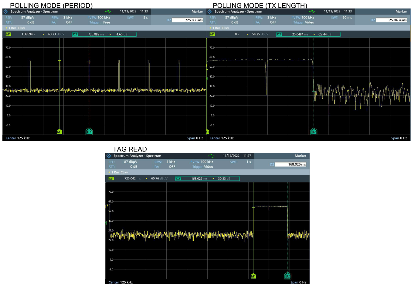
Figure 7: Example Pulsed Emission Characteristics (Duty Cycle).
