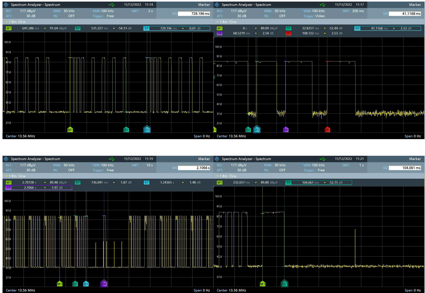
Figure 7: Example Pulsed Emission Characteristics (Duty Cycle).
