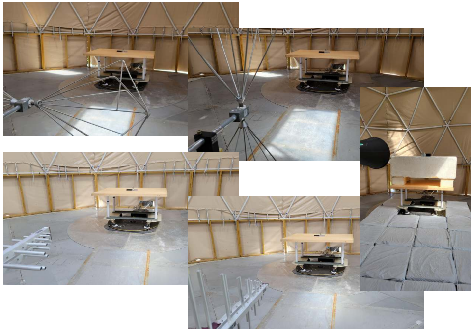
Figure 4.1.1 (v) Radiated Emissions Test Setup Photograph(s).
