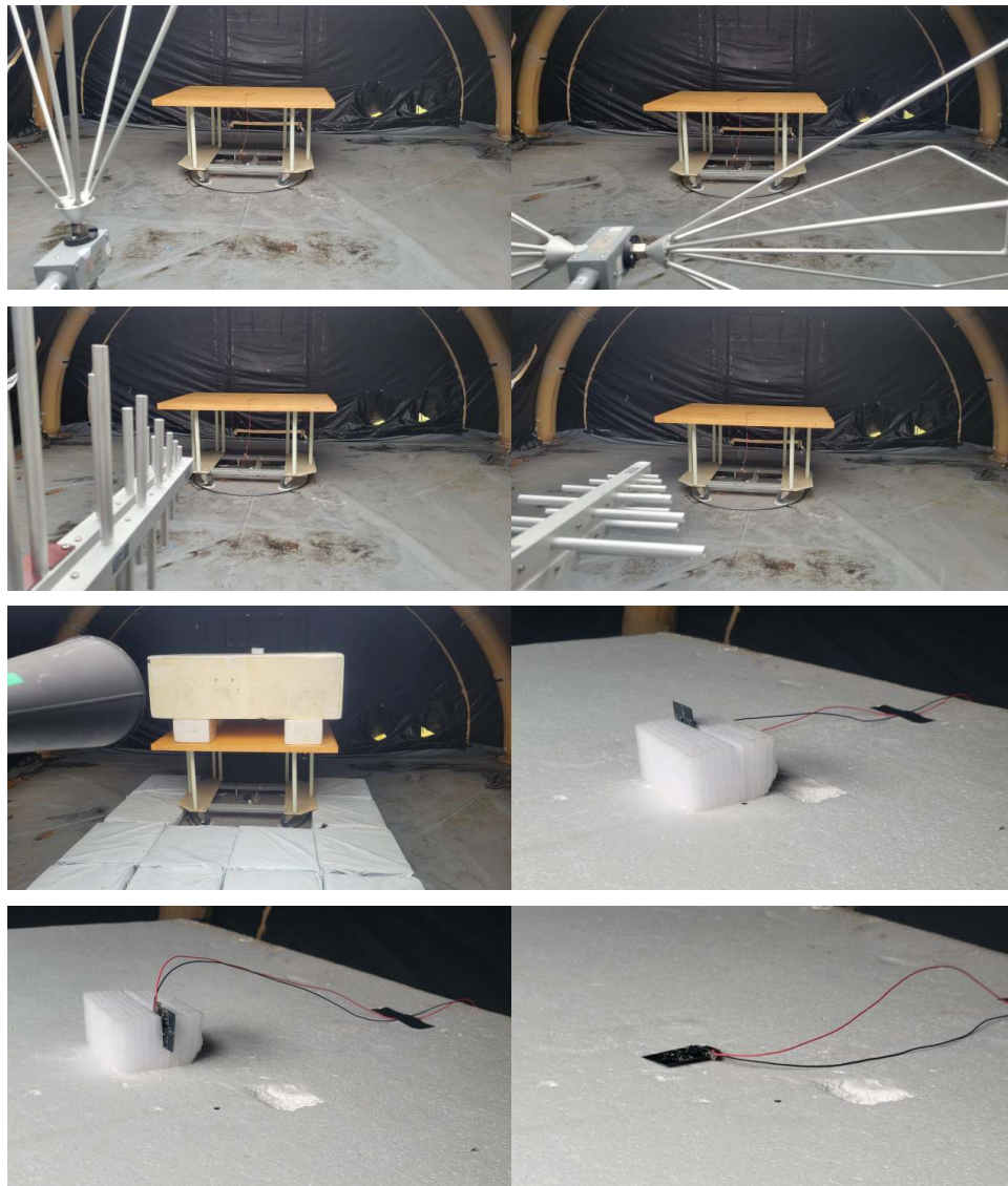
Figure 4: Radiated Emissions Test Setup Photograph(s).
