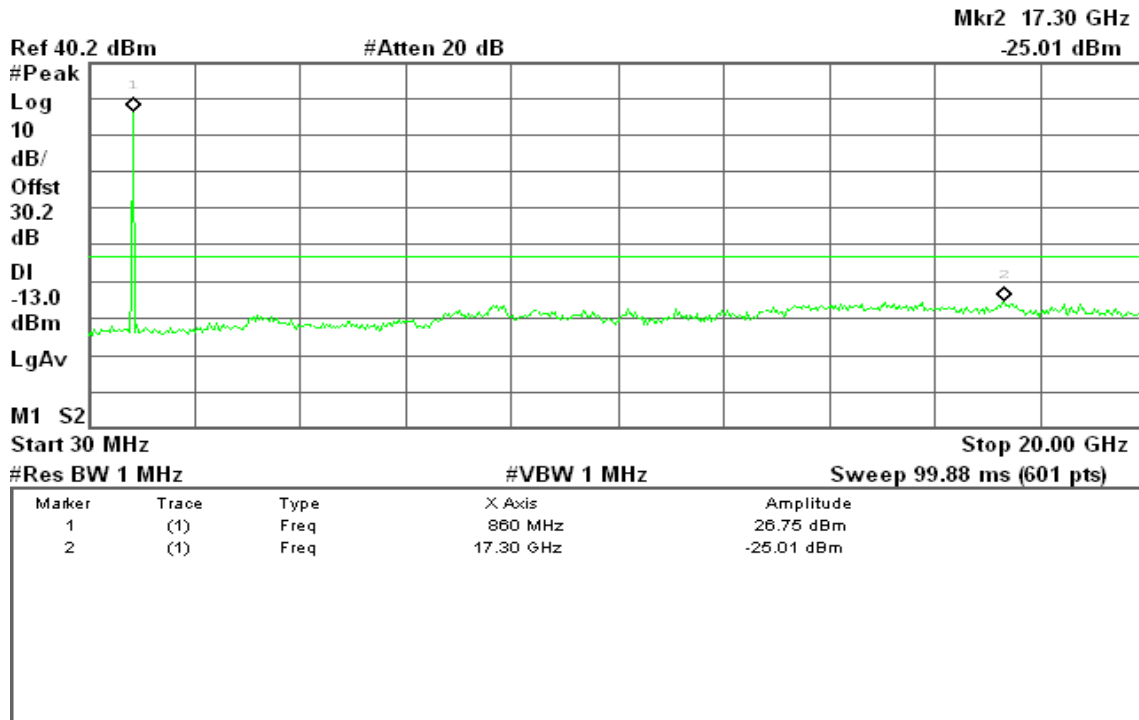
Figure 8-3: Out of Band emission at antenna terminals – CDMA2000 1xEVDO / CH High
