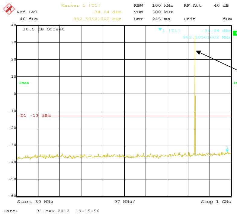
Fundamental test with Band Reject Filter
