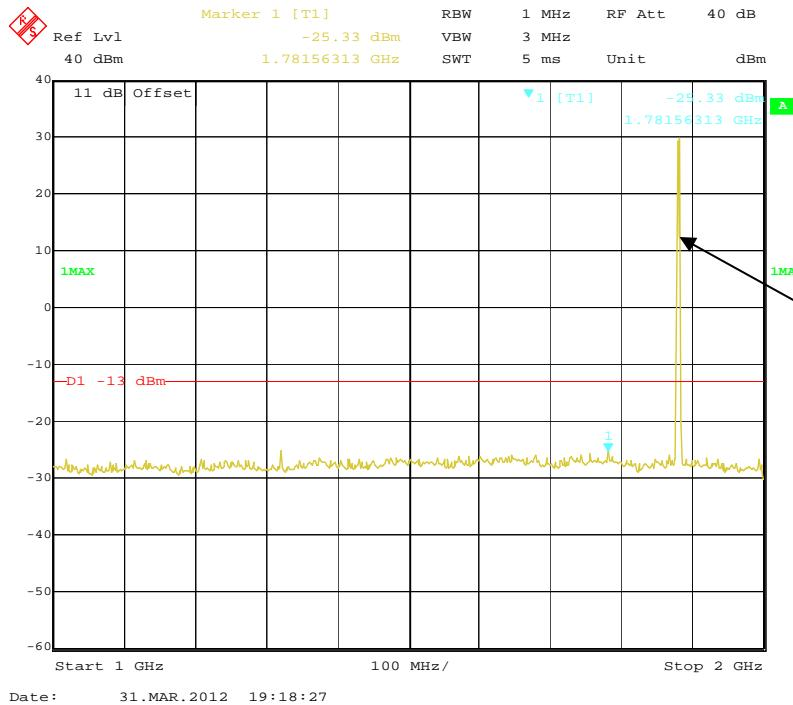
Fundamental test with Band Reject Filter
