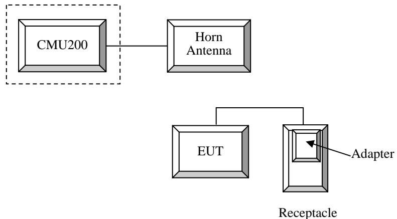
**Block Diagram of Test Setup**
