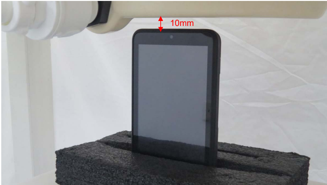
Picture 5: Top Side, the distance from handset to the bottom of the Phantom is 10mm
