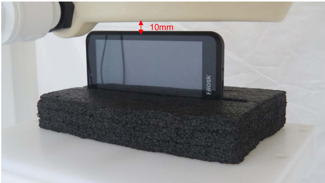
Picture 4: Right Side, the distance from handset to the bottom of the Phantom is 10mm
