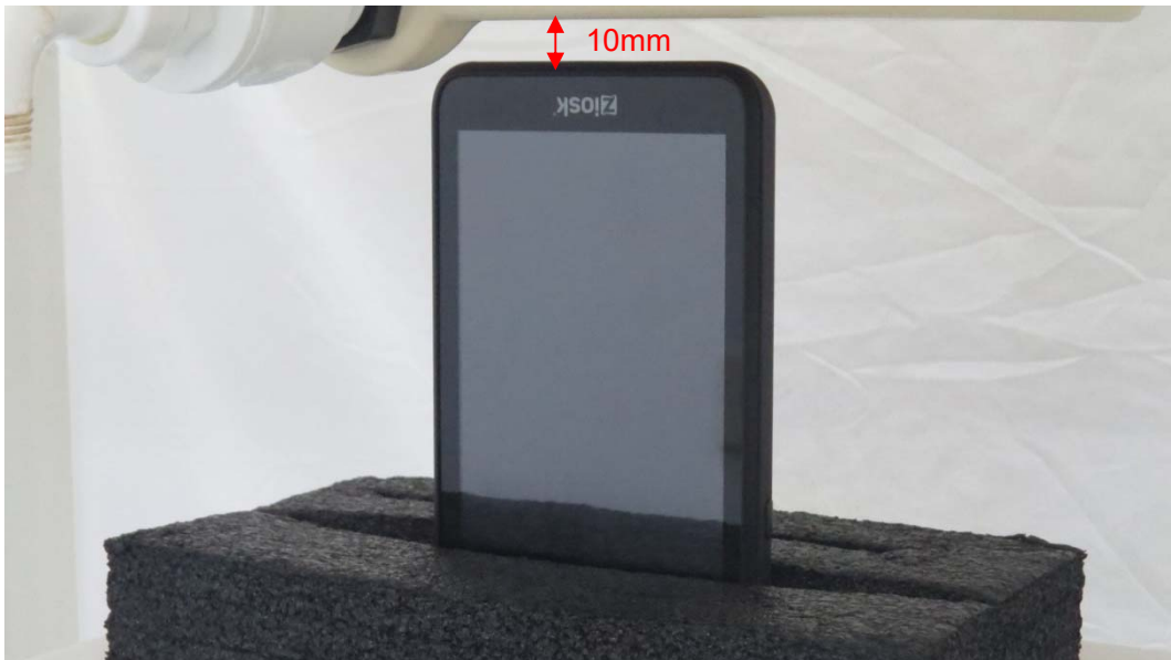
Picture 6: Bottom Edge, the distance from handset to the bottom of the Phantom is 10mm
