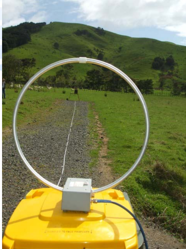
Small Antenna at 30 metres (White line is the tape measure)
