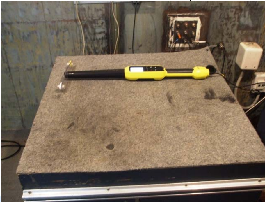
Conducted emissions test set up
