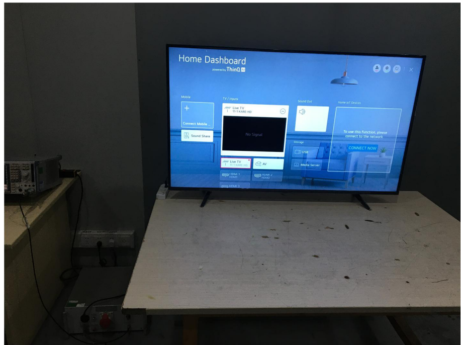
Conducted Emission Test Setup
