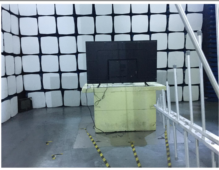
Radiation Emission Test Setup (30MHz to 1GHz)
