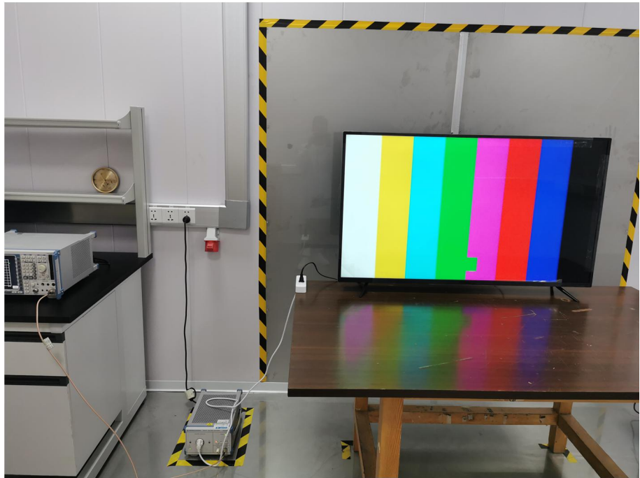
Conducted Emission Test Setup
