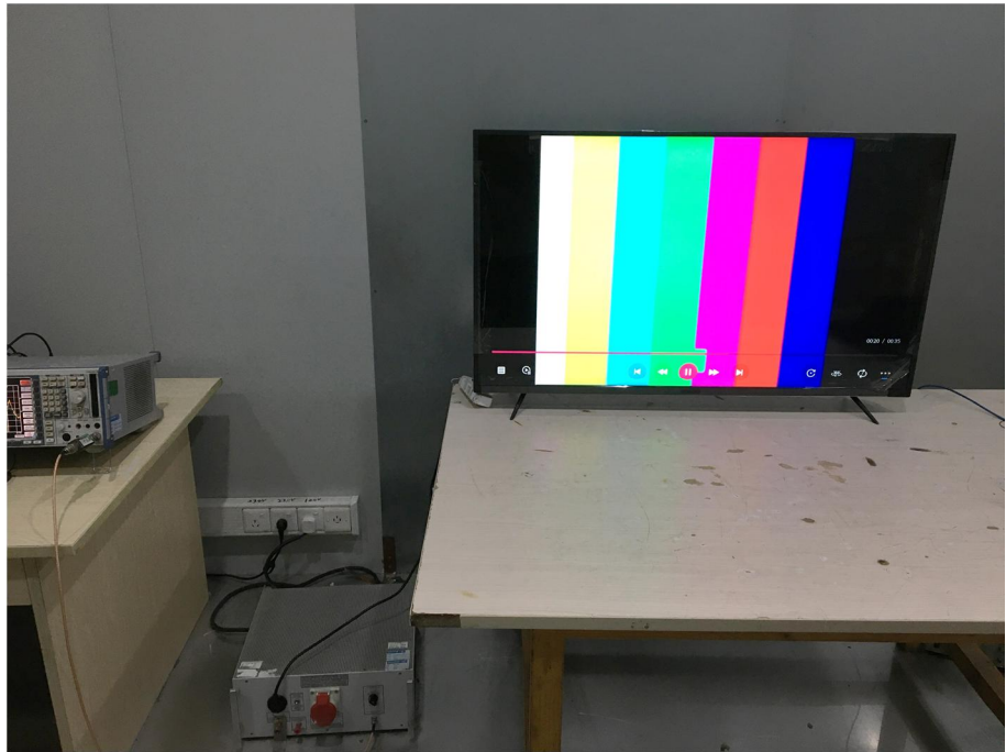
Conducted Emission Test Setup
