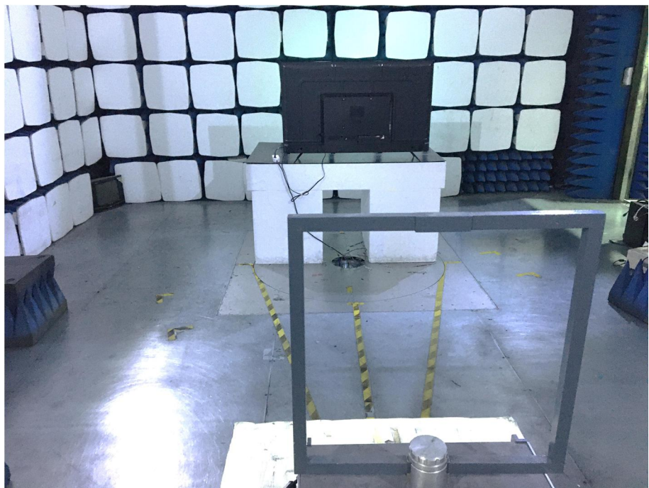
Radiation Emission Test Setup (Below 30MHz)
