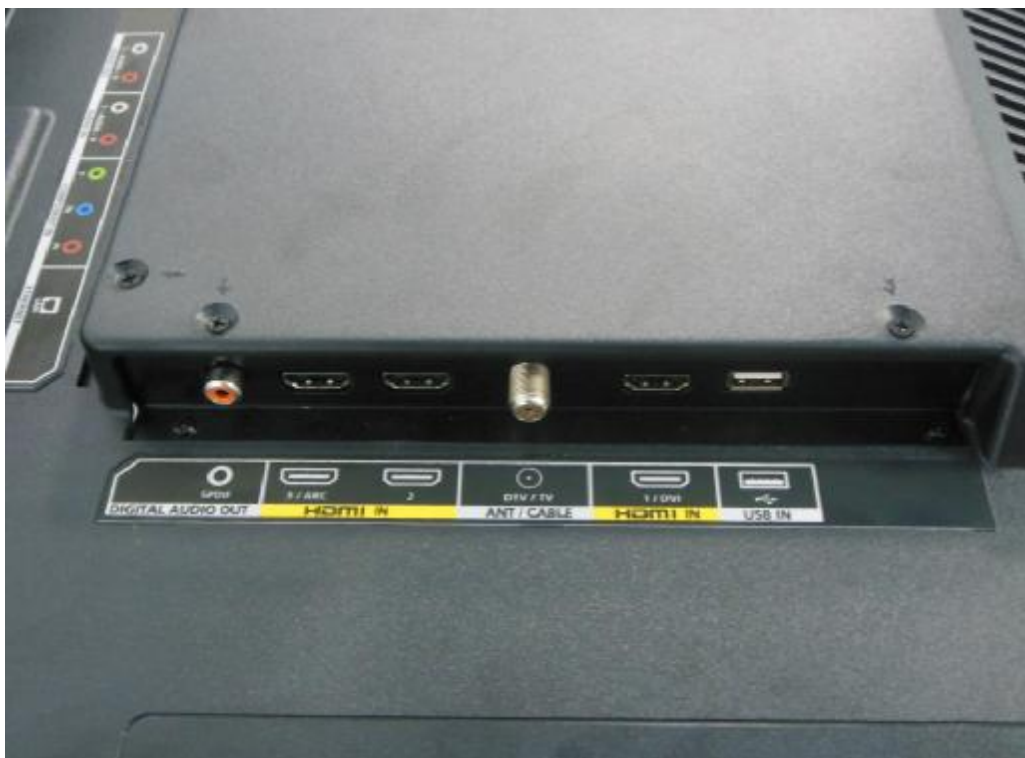
EUT – Port View
