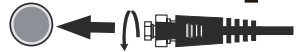
Satellite, cable or TV antenna cable to TV ANTENNA terminal (cable not included)
