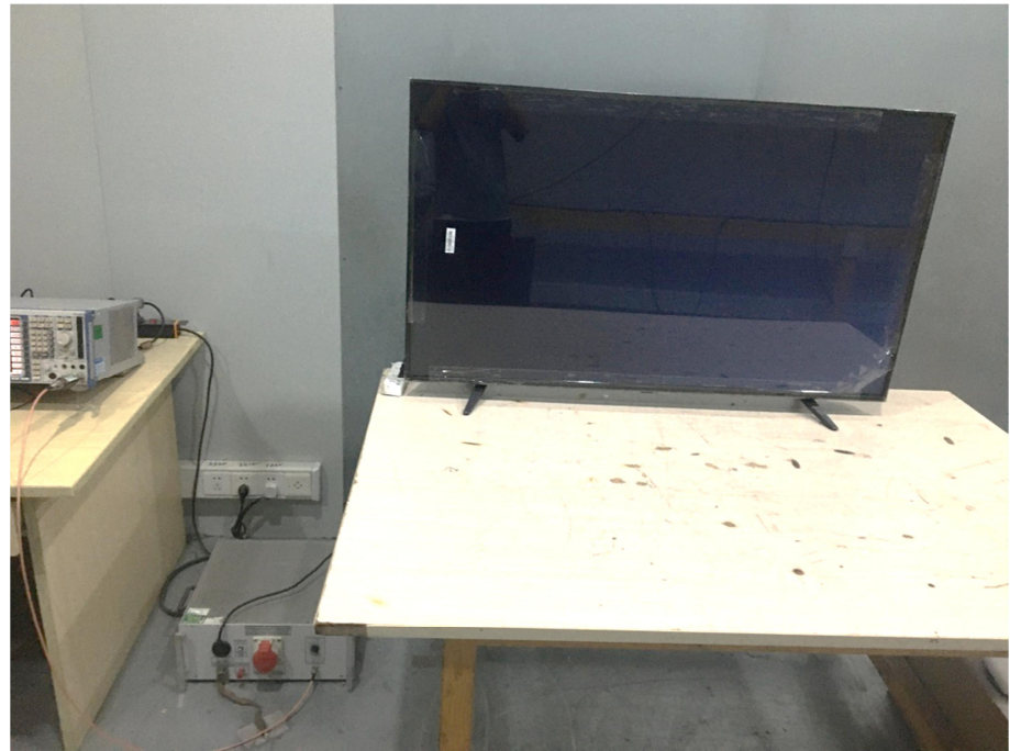
Conducted Emission Test Setup
