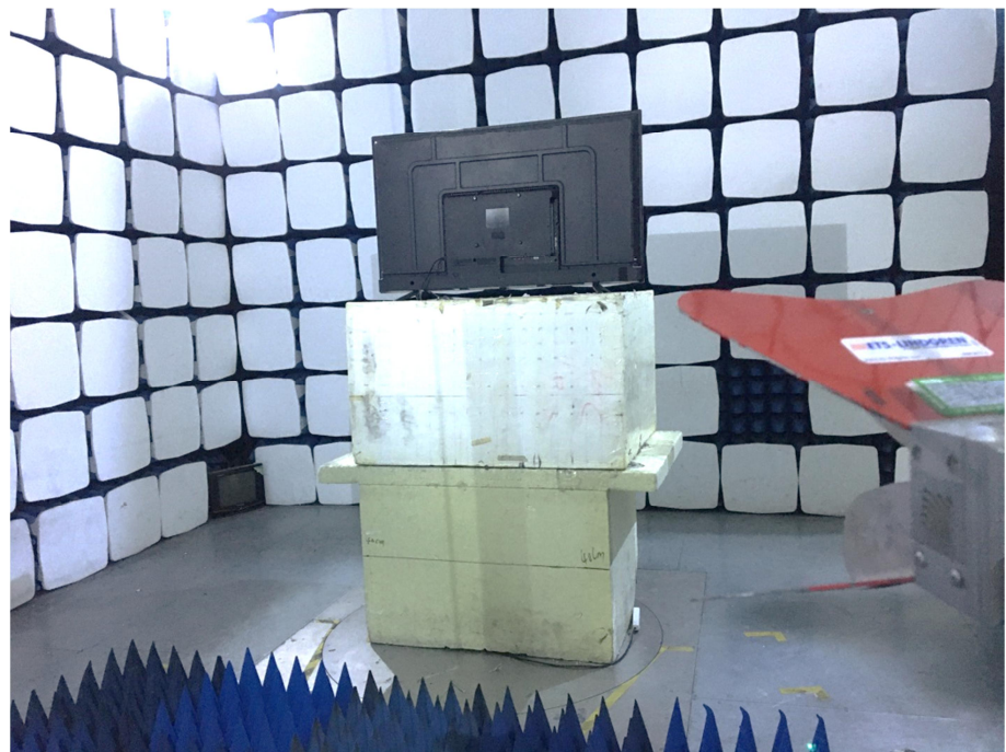
Radiation Emission Test Setup (1GHz to 18GHz)
