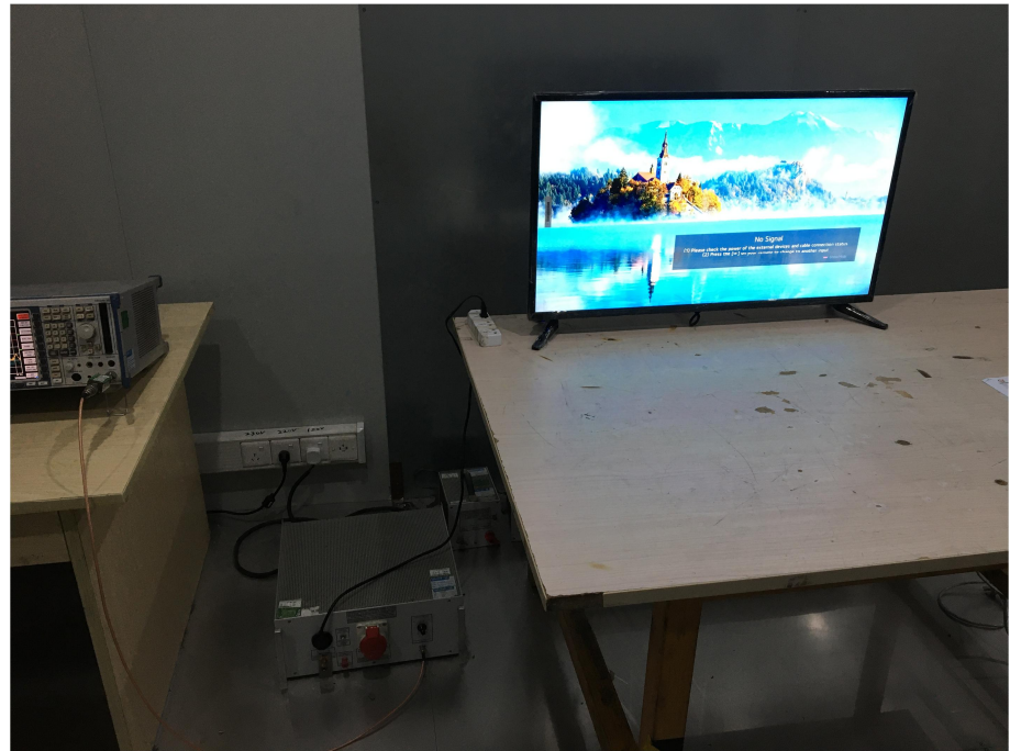
Conducted Emission Test Setup
