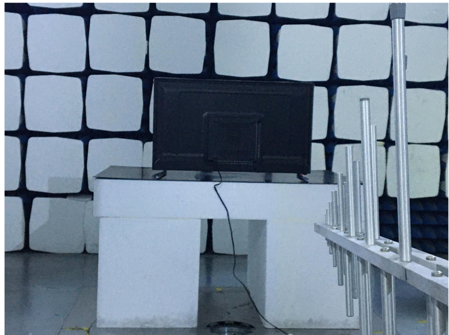
Radiation Emission Test Setup (30MHz to 1GHz)
