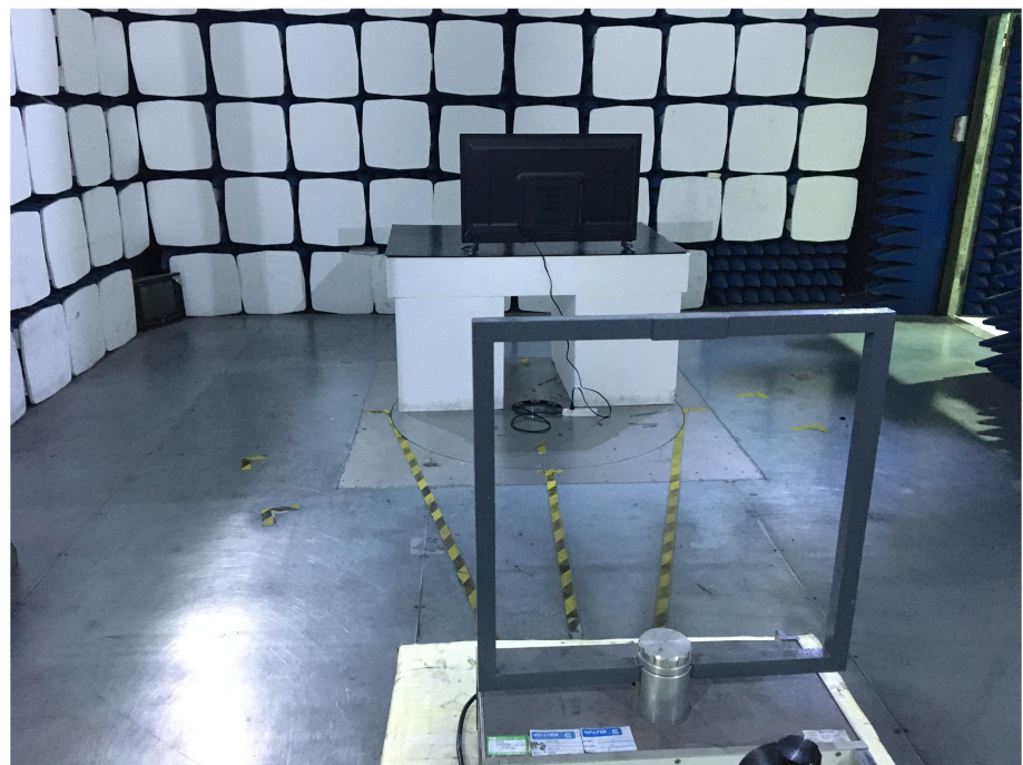
Radiation Emission Test Setup (Below 30MHz)
