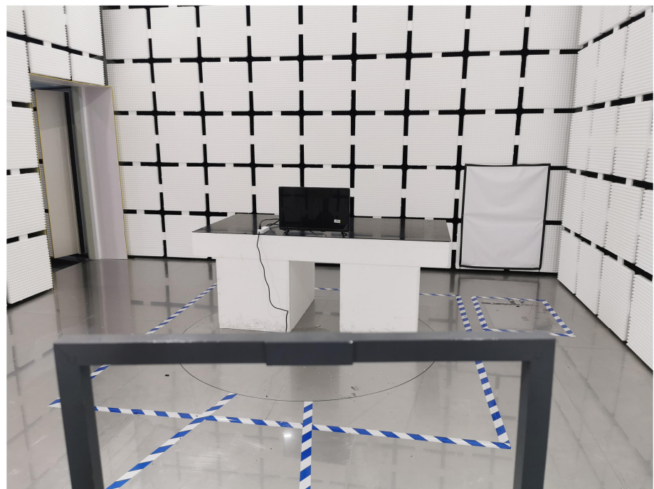
Radiation Emission Test Setup (Below 30MHz)
