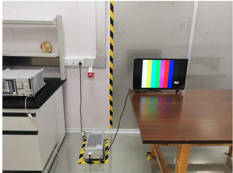
Conducted Emission Test Setup
