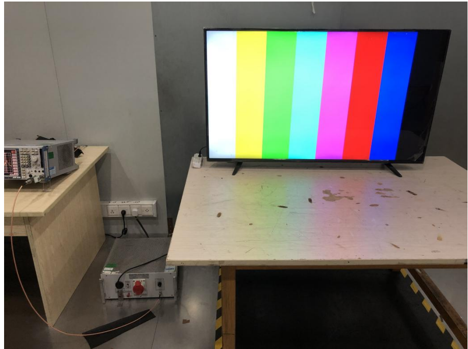
Conducted Emission Test Setup
