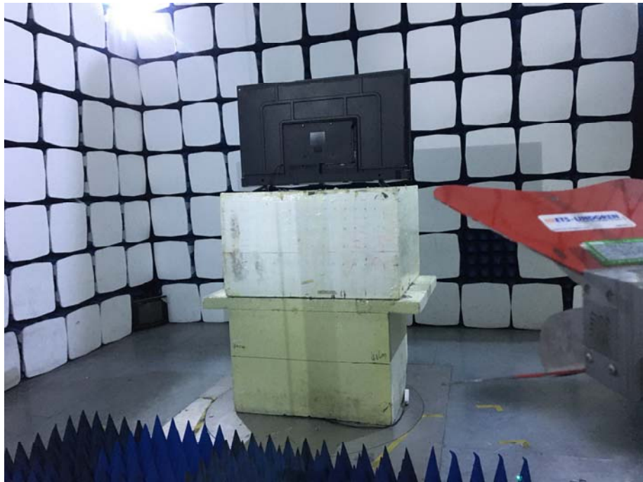
Radiation Emission Test Setup (1GHz to 18GHz)
