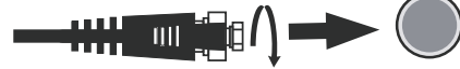
Satellite, cable or TV antenna cable to TV ANTENNA terminal (cable not included)
