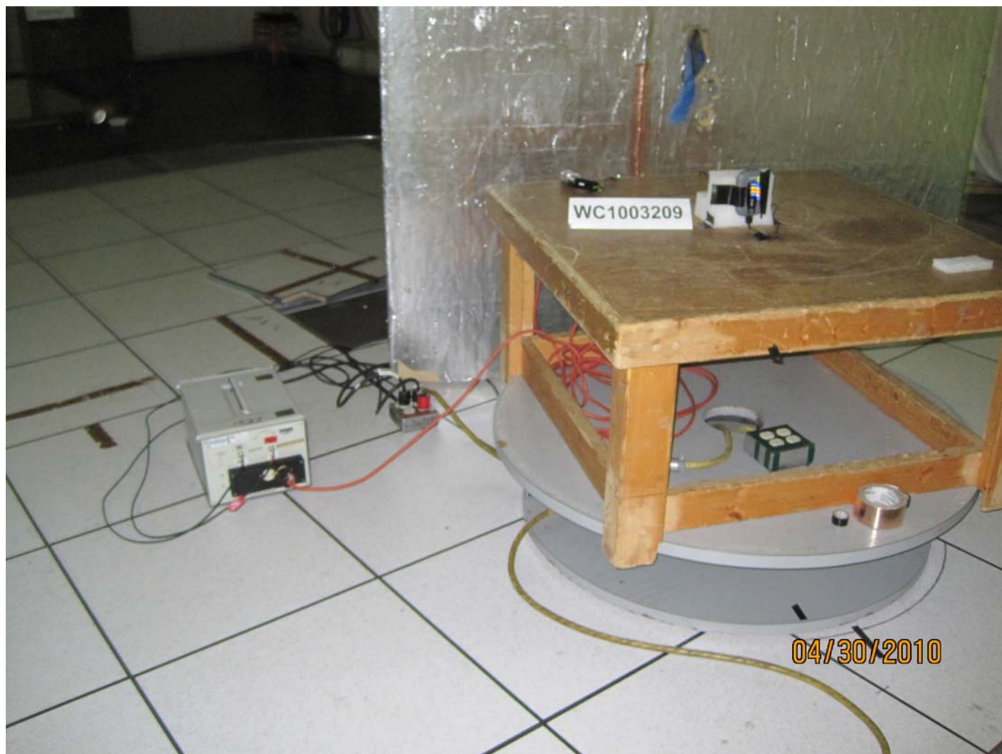
Test-setup photo(s): Conducted emissions
