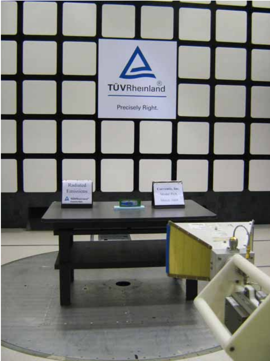
Figure 3: Photo of Test Setup for PiiX, 1GHz to 18GHz (Front View)
