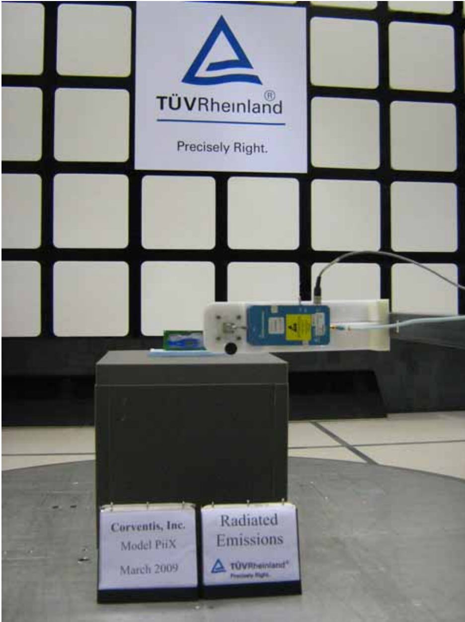
Figure 5: Photo of Test Setup for PiiX, 18 GHz to 26GHz (Front View)
