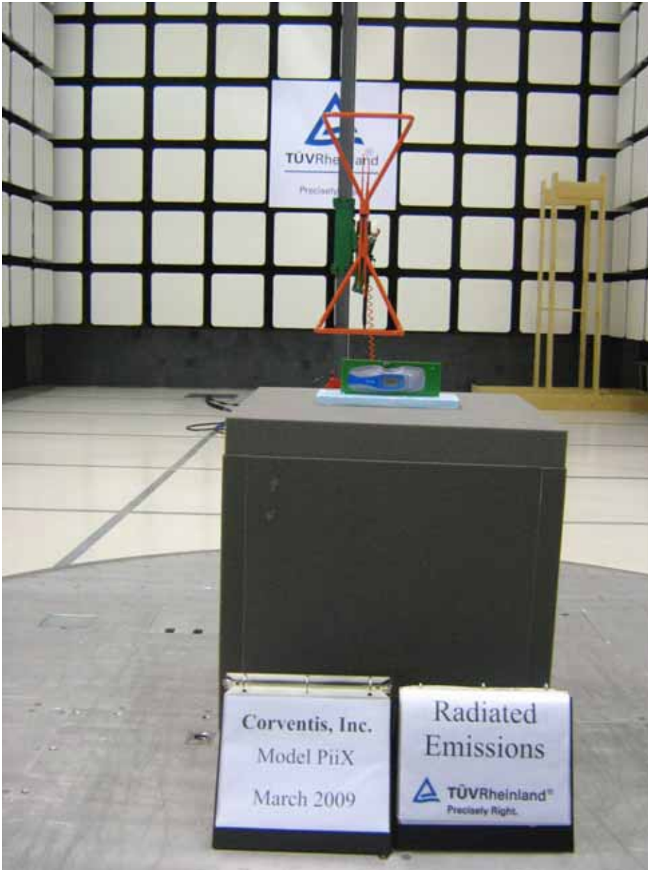
Figure 2: Photo of Test Setup for PiiX, 30 to 1000 MHz (Rear View)
