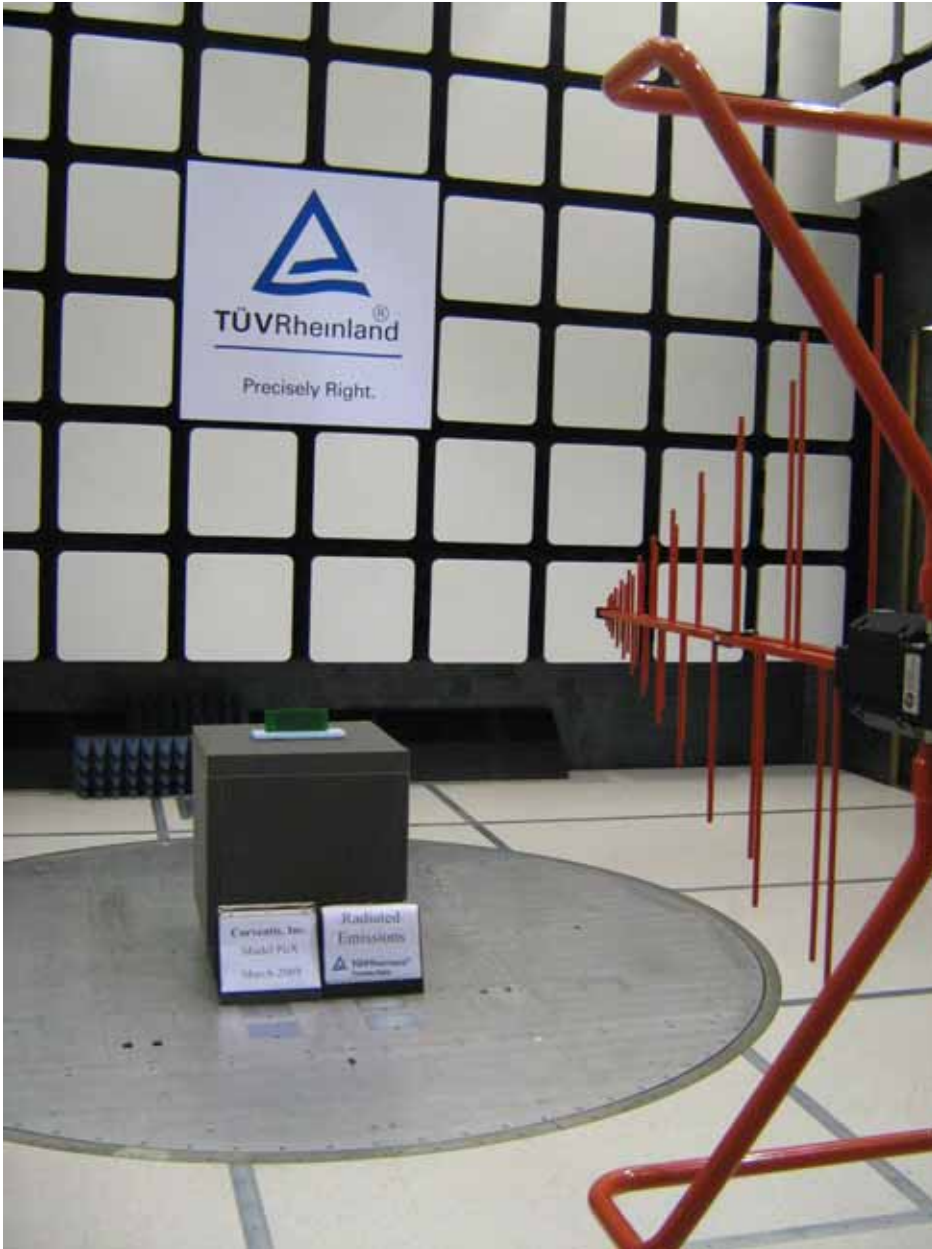
Figure 1: Photo of Test Setup for PiiX, 30 MHz to 1000MHz (Front View)
