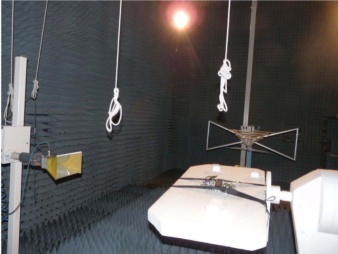
Photo 3: Test setup for radiated measurements (Enclosure, IC RSS-Gen: above 1 GHz, FCC: above 30 MHz)
