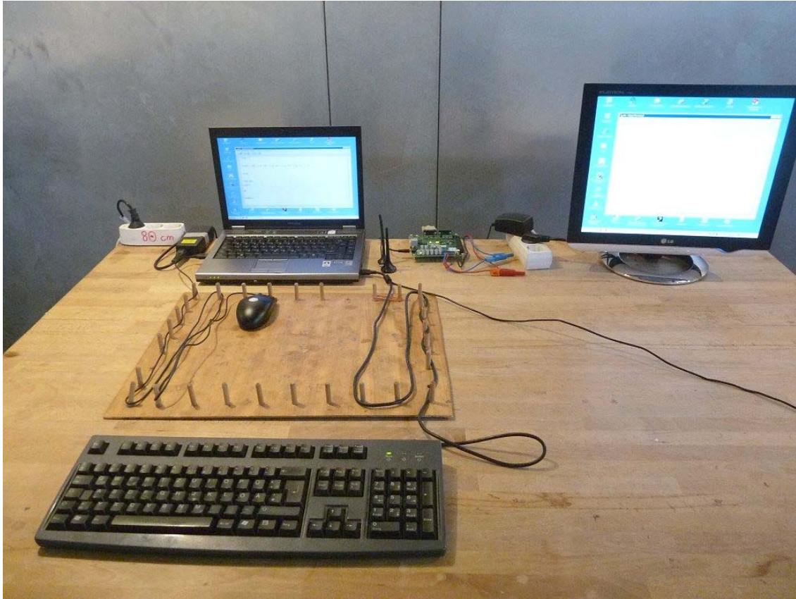
Photo 5: Test setup for conducted measurements (connected to AC Mains via AC/DC adaptor, measured at PC, computer peripheral setup)
