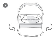
Turn the Feeder upside down to access the battery compartments.
