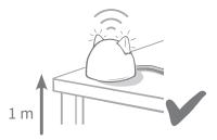
Place the Hub at least 1 metre off the ground (i.e. on a table that is as clear of obstructions as possible).
