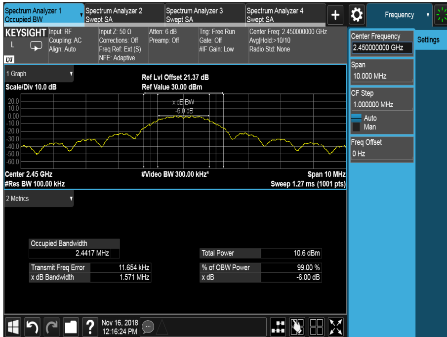
Figure 40 - 2450 MHz – 6 dB Bandwidth and 99% Occupied Bandwidth
