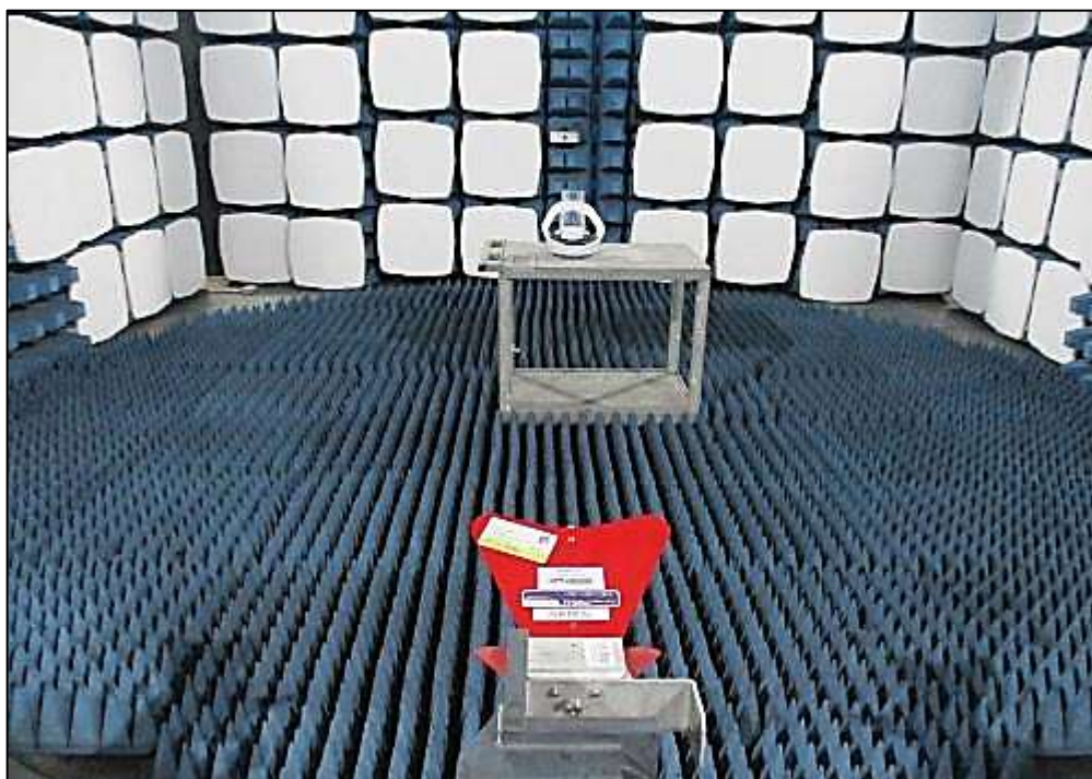
Figure 15 - Test Setup - 1 GHz to 13 GHz
