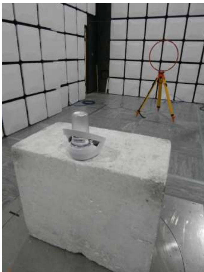
Figure 12 – 9 kHz to 30 MHz – Semi Anechoic Chamber
