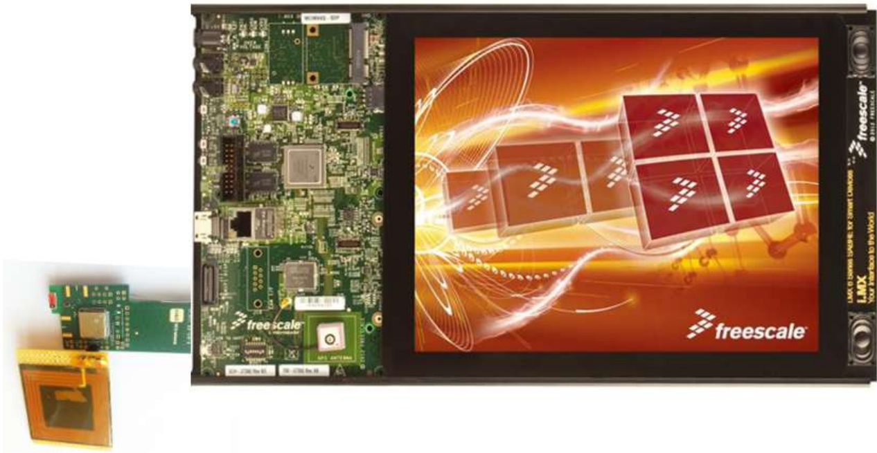
The SPB209A-EVK with SPB209A module and a custom NFC antenna connected to a i.MX6 DL Linux Host Platform.
