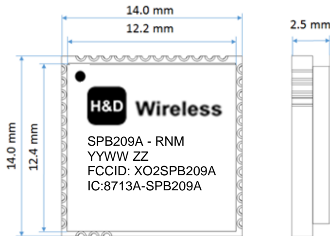
Figure 2.1: Mechanical drawing, equivalent to a 41 pin Quad Flat No-Lead (QFN) package.
