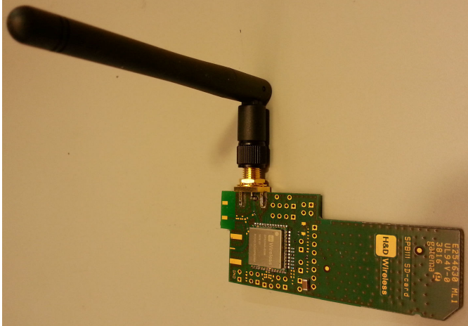
Figure 5, SD-card SPB111 with module SPB209A using Walsin RFDPA870900SBLB8G1 antenna.
