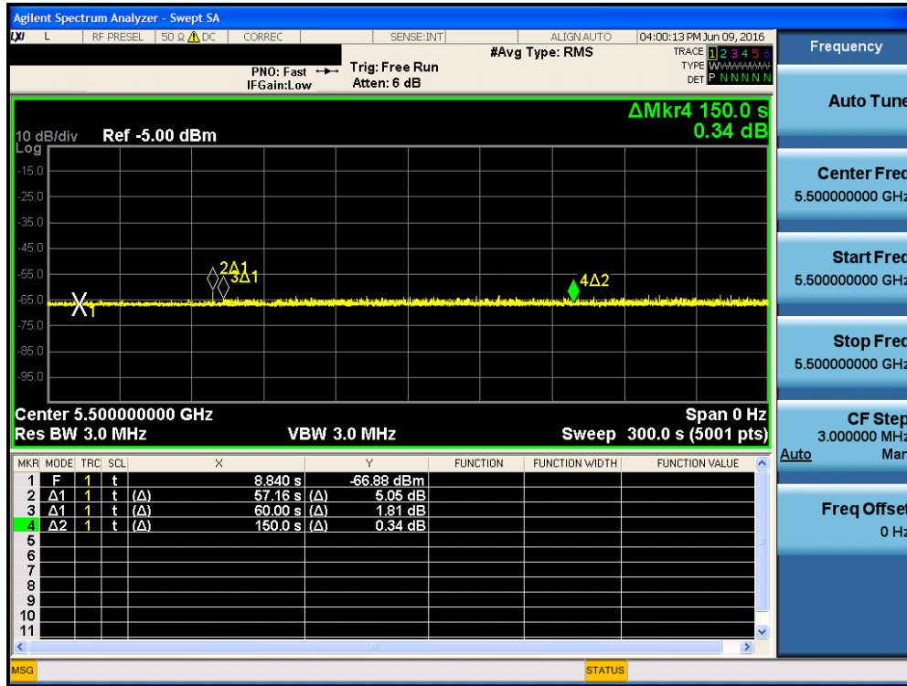
Plot 5-16. Radar Burst at End of CAC Time
