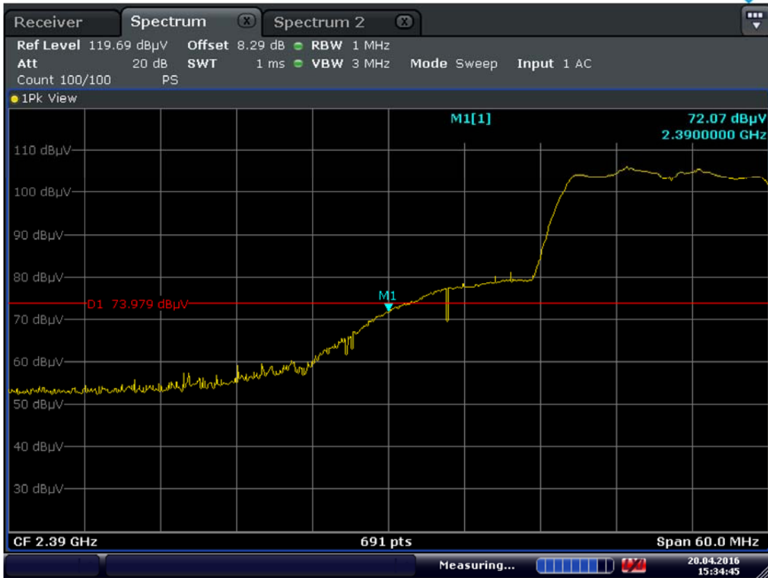
Plot 7-52. Radiated Restricted Lower Band Edge Measurement (Peak)
