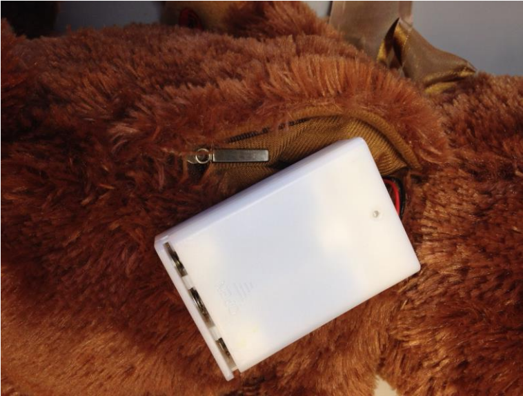
Figure 4: Battery box accesible via zipper.
