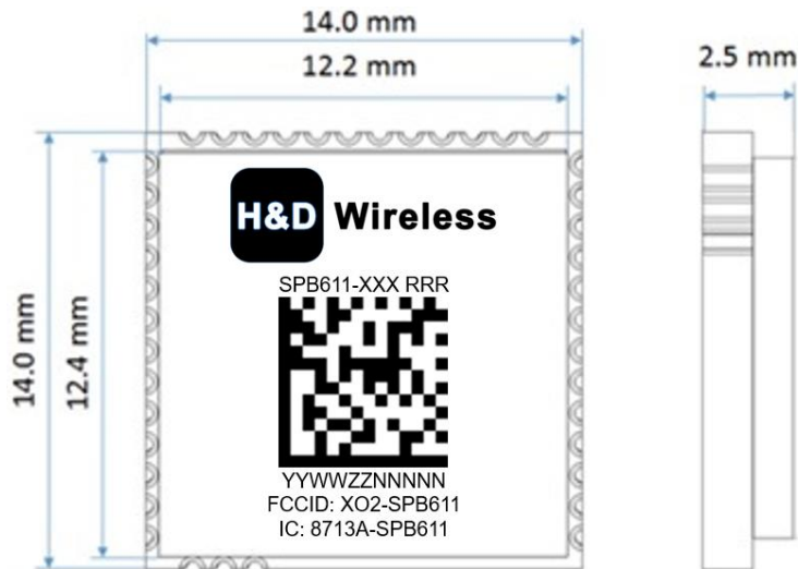
Figure 1, Mechanical drawing, equivalent to a 41L QFN package. N.B. Drawing not to scale.
