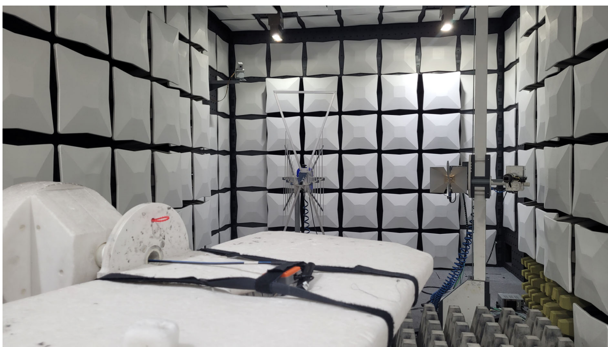
Photo 4: Test setup for radiated measurements above 1 GHz
