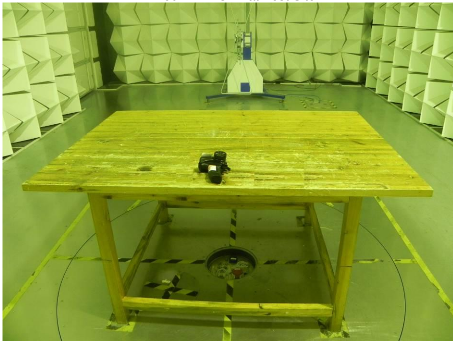
30MHz-1GHz at Test Site 2#
