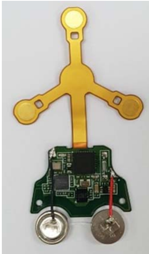
Internal - PCB and Batteries
