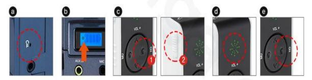
If wireless connection is not qualitativelyWhen you use a new wireless microphone, you can easily re-register and use it.
