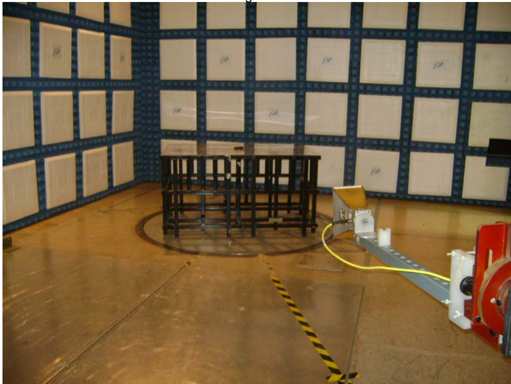
Test Setup for Radiated Emissions – Horizontal Polarity above 1000MHz
