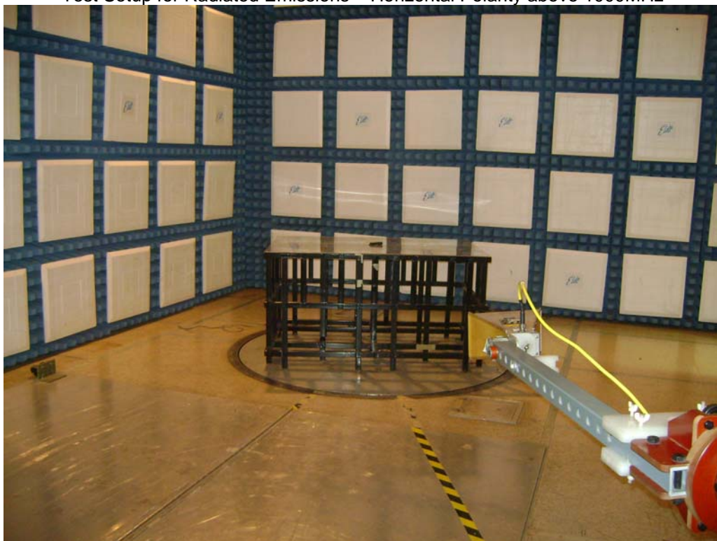
Test Setup for Radiated Emissions – Vertical Polarity above 1000MHz
