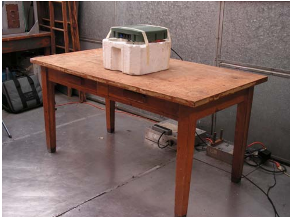
Photograph 6.9. Close-up of DUT on Conducted Emissions Table (Class A verification)
