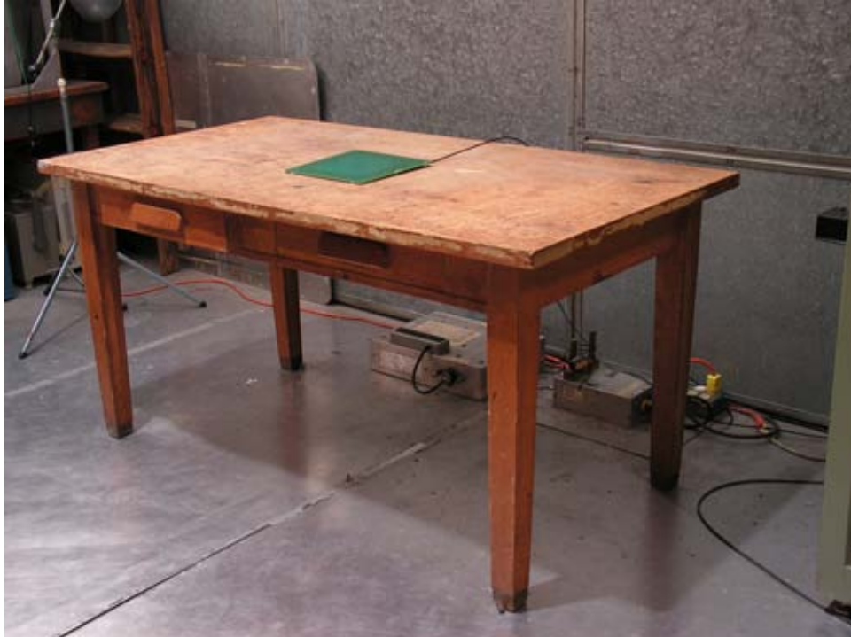
Photograph 6.8. Close-up of DUT on Conducted Emissions Table (Class B transceiver verification)
