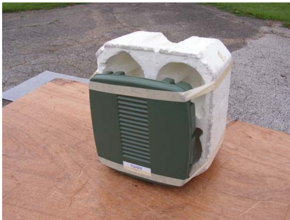
Photograph 6.7. Close-up of DUT on OATS (one of three axes tested)
