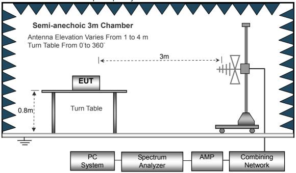
(B) Radiated Emission Test-Up Frequency Above 1GHz
