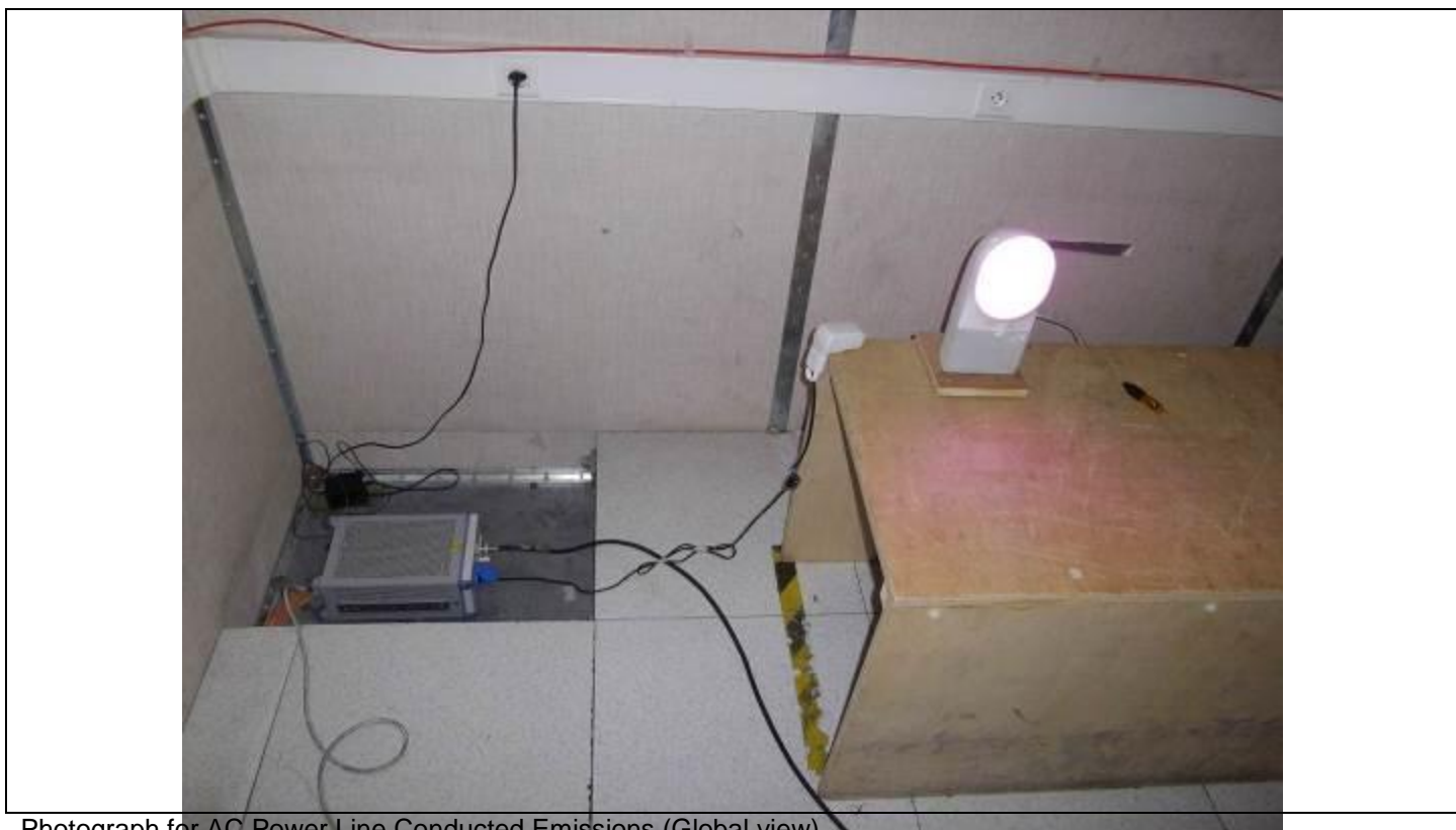
Photograph for AC Power Line Conducted Emissions (Global view)
