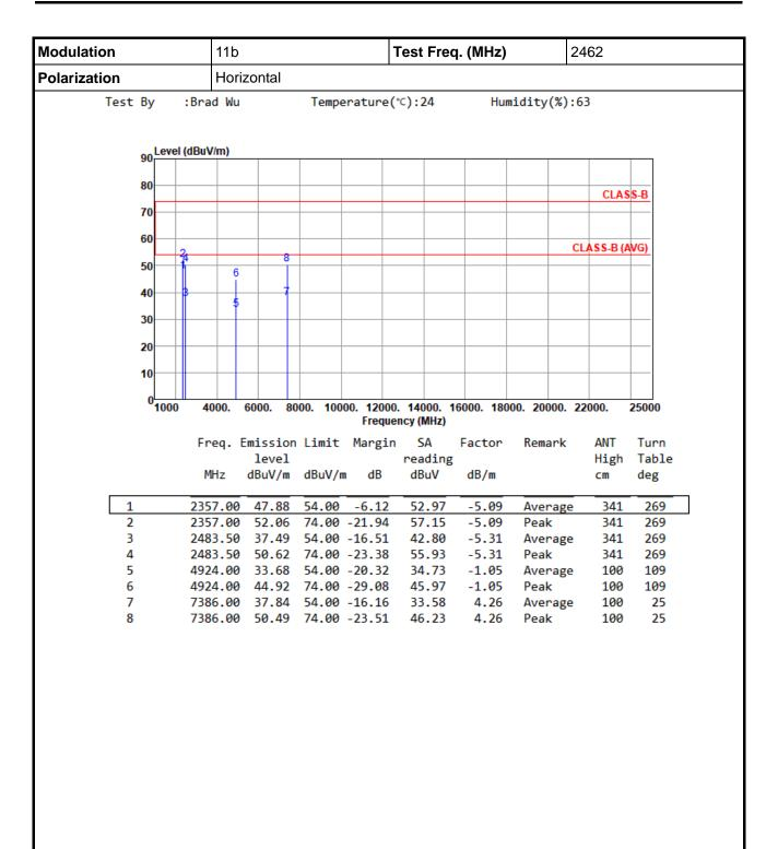
\*Factor includes antenna factor, cable loss and amplifier gain
