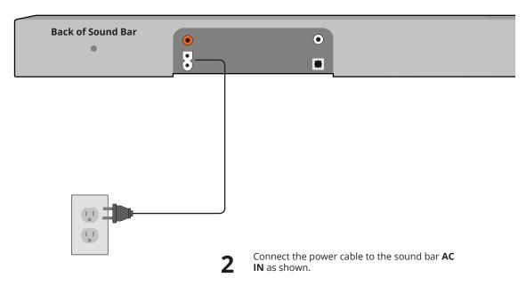
Plug the power cable into an electrical outlet.
