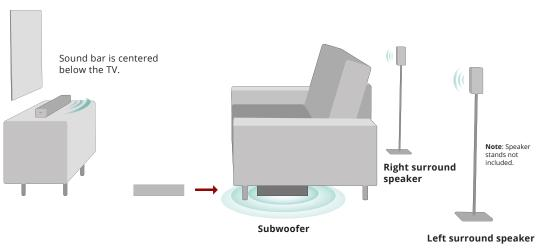
**Note**: Do not block the subwoofer port. Port should be facing the front of the couch.
