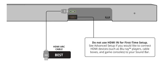
HDMI cables send Video (Out) and receive Audio from the TV/Display.
