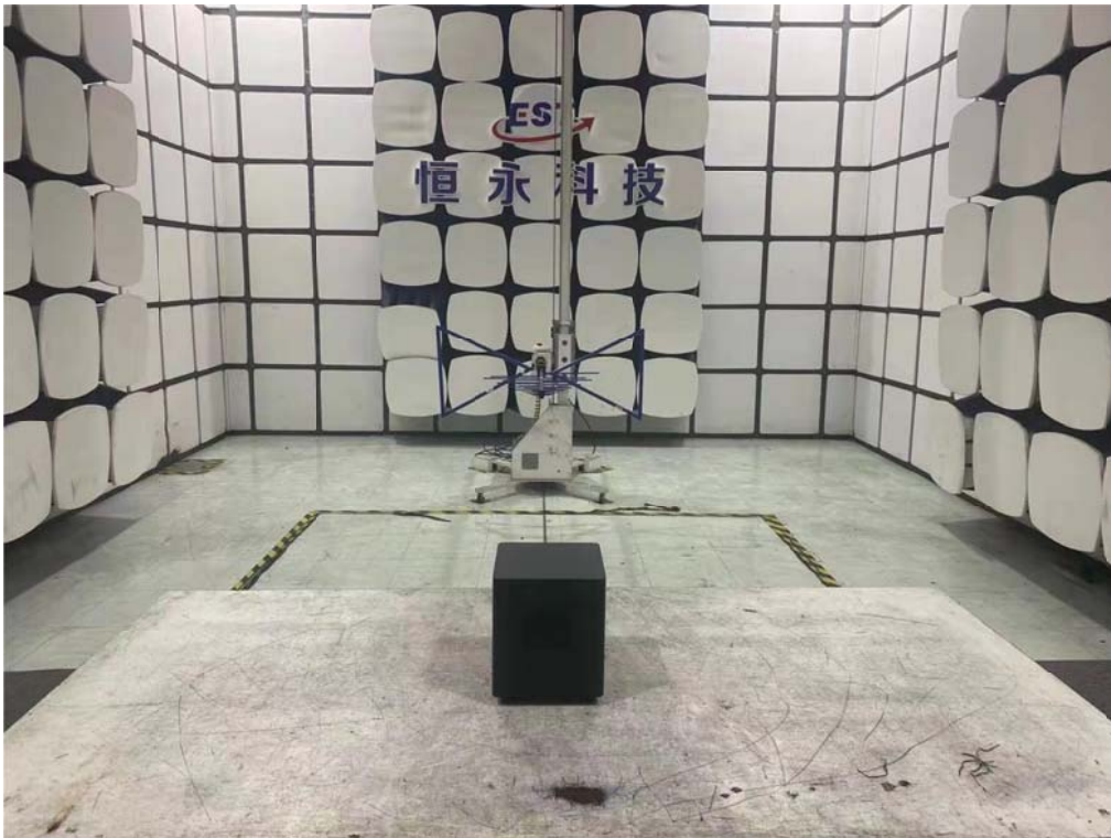
Radiated Test (30-1000 MHz)
